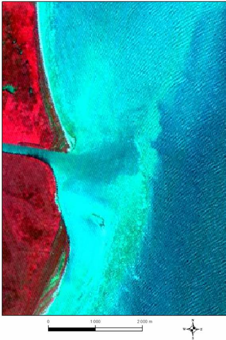
Simulated field of suspended sediments ( d=0.02 mm) for the conditions of South-East- South waves and the satellite picture Terra (ASTER) 12.01.2001, which presents the image of river muddy water in the sea under the impact of South- East waves
